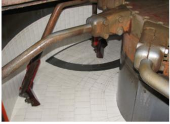
ALOTEC ceramic linings have proven to be effective for virtually all makes and types of agitator. The high wear resistance of the material ensures long life and increased efficiency.
